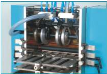
Roller gap adjustment by Calipers
